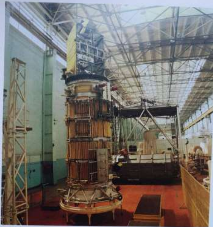
120. SM-K space apparatus used for studying the Sun and its particles
